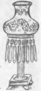
THE SOLAR LAMP was patented in Philadelphia in 1843. Similar to the Argand and the Astral, with the wick closely fitted into a round tube that extended through the bottom of the oil font—an inverted bell shaped reservoir. The Solar had a bulb-shaped chimney. Like the Astral, they were usually graceful with brass or bronze columns rising from a pedestal base.
