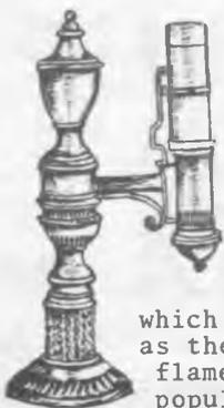
THE FIRST REALLY NEW IDEA in lighting devices was the Argand lamp. In 1783 a Swiss chemist, Aime Argand, invented a lamp that increased the draft and made the flame brighter—equal to ten candles. The Argand lamp burned vegetable or whale oil. It had a cylindrical wick that admitted air on both the inside and the outside of the burner, which made the light brighter as well as the glass chimney that held the flame steady. The Argand became very popular although never inexpensive.
