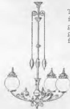
The most commonly used gas fixture was the gasolier--or gas chandelier. Clear glass globes were seldom used for gas fixtures. Kerosene lamps had often used clear glass chimneys so as not to diffuse its relatively feeble light, but the higher candle power of gas light caused glare. So domes, shades and globes were colored, frosted, milk and egg
